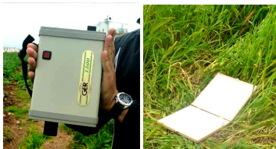
Fig. 5. GER 1500 used in this study with its calibration target
