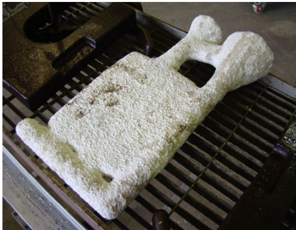
Fig. 15. The last coarse ceramic coating forming the final shell with the casting feeder and air evacuation cones and tubes
