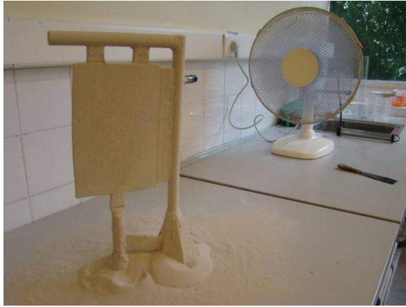
Fig. 14. The first silica-sand ceramic thin layer recovering the wax replica
