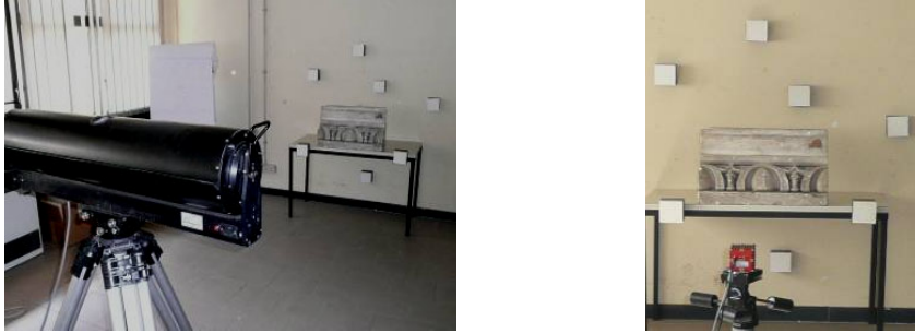
Fig. 1. The MENSİ S10 and SR-4000 camera record the decoration
