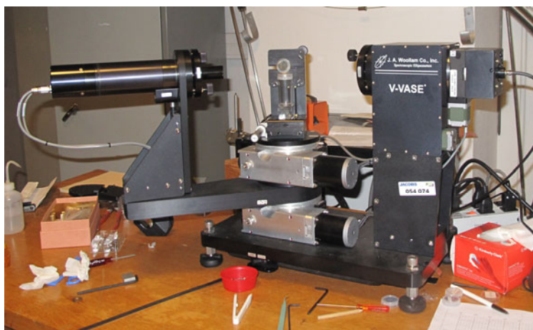
Fig. 11. The Woollam Ellipsometer used for optical constants acquisition ( n and \kappa ) at INSP (Paris)
