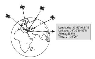
Figure 1: The basic function of satellite navigation
