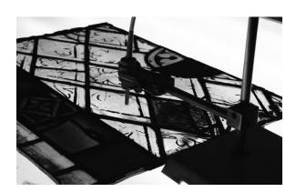
Figure 9: The stained glass window part studied in spectrophotometry. The work dating from the XIVth century isdeposited for restoration. It exhibits few colored peripheralregions only.
