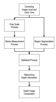
Figure 1: Processing flow diagram of retouching method
