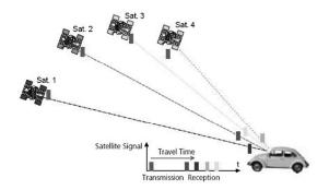
Figure 2: Four satellites are needed to determine Longitude, Latitude, Altitude and Time
