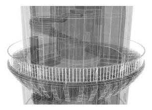
Figure 4: A partial view of a 3D model of the signal light tower, showing the balcony on level 3 and the spiral staircase (UMR MAP, 2006).
