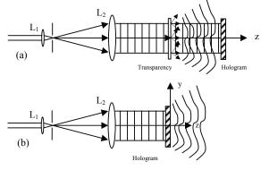
Figure 1: Gabor's on-axis optical configuration to a) record a wave field and b) reconstruct it without need of the actual object. (L<sub>1</sub>, L<sub>2</sub> Lenses)
