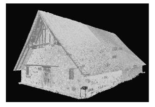
Figure 9: The complete point cloud of the Church of Podithou
