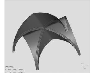
Figure 7: Vaulting prepared based on survey. Software: 3DMAX, edited by Geomagic Studio
