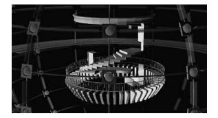
Figure 5: A view from the inside of the signal light tower, showing the spiral staircase and the balcony on level 3 (UMR MAP, 2006).
