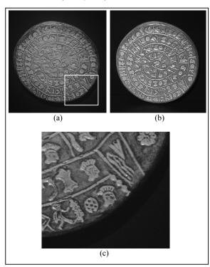
Figure 4: Photos of a reflection hologram of a "Phaestos Disc" copy, recorded by a cw green laser (at 532nm). (a) Front view, and (c) detail of the same hologram, marked with red in (a). (b) Photograph of the copy under white light.
