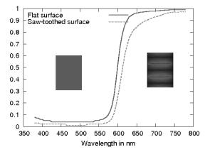
Figure 2: Reflectance factor of two samples of a cinnabardry paint film. The visual difference between a flat sampleand a saw-toothed surface is shown. The saw-toothed sample surface will appear darker and brownish-red compared to the flat sample placed in the same lighting and viewing conditions. The small included pictures of the physical samples are superimposed beside the correspond cures.
