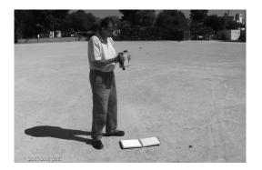
Figure 2: Collection of spectral signature data on a whitish bare soil using the GER1500 Field Spectroradiometer
