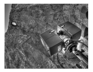
Figure 1: During the survey of the so called "Serapeo" in Villa Adriana, Tivoli (near Rome), the double scans for each scanner station done (the first at high and the second at low resolution) allowed to produce a double pointcloud to better fit the different purpose of data treatment.
