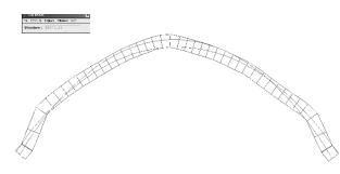
Figure 7: Minimum and maximum thrust for the example vertical section 1\_11
