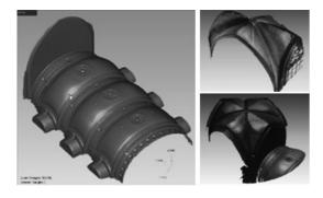
Figure 5: Meshed models of the vaults of the St. James church
