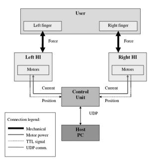
Figure 1: Haptic System diagram
