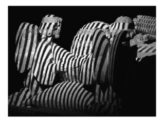
Figure 3: Digitization of the recumbent shape using a structured light device.
