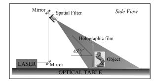
Figure 2: Side view of a single beam set up for the recording of a reflection hologram
