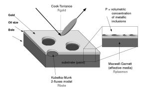
Figure 4: The physical description of the optical interactions accounted for the rendering of a gold leaf deposited n a colored bole. Small cracks due to the application process and the natural holes in thin metallic films are described. Their surfacic density creates a diffuse contribution to the reflected light.
