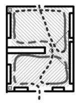
Figure 8: Overlapping camera zones in a multi entry room
