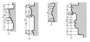
Figure 7: Profiles got from point cloud.
