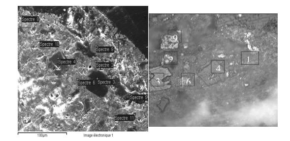
Figure A4: SEM image (left) indicating the identification points where the spectra were recorded. The right optical image is a vertically symmetrical view of the SEM image.
