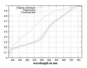
Figure 3: Comparison of two normalized spectrophotmetric measurements made on the bluish regions. The normalized diffuse reflectance factors show the background influence on the paint appearance. The blue pigments were deposited on the brownish colored preparation. All the colors of the work are influenced by this colored underlayer. Top curve: original blue.
