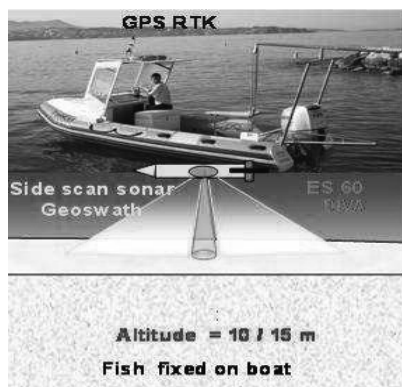
Figure 5 shows principles of multisensor acquisition in shallow water on the SEMANTIC survey boat.
