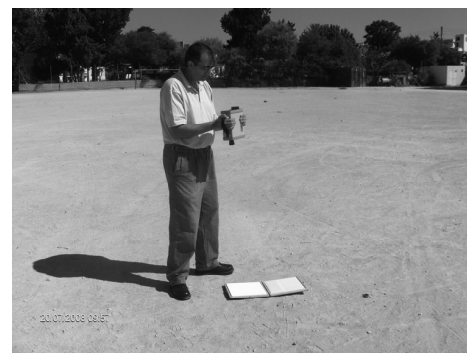
Figure 5: Collection of reflectance measurements on a whitish bare soil using the GER1500 Field Spectroradiometer and the Spectralon™ White Panel.
