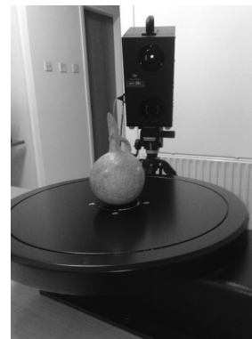
Figure 1: The scanning setup. We can see the 3D scanner, the rotating stage and the artefact.
