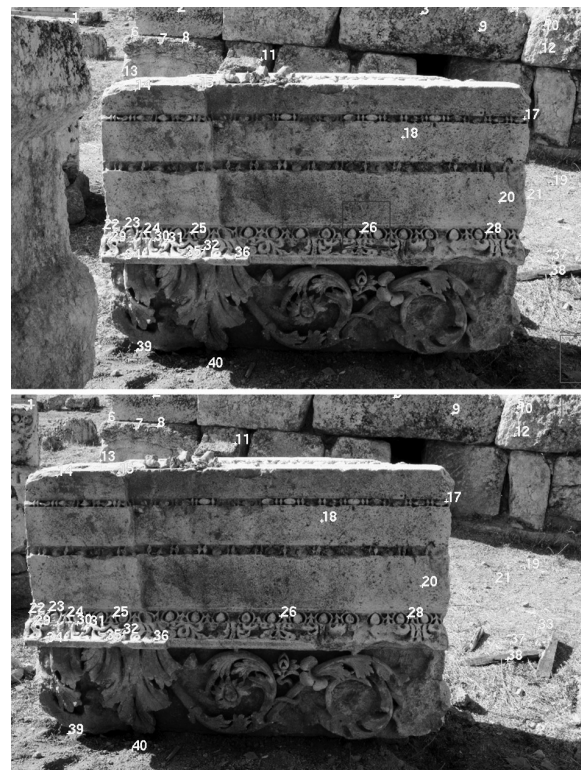
Figure 4: Homologous image points, extracted using Förstner-Operator, followed by cross-correlation
