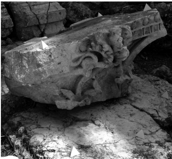
Figure 3: Using white tetrahedra as 3D targets for the linkage of several stereo models
