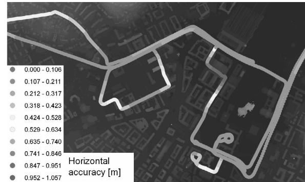
Figure 6 : Estimated horizontal accuracy of the trajectory after GNSS/IMU post processing.
