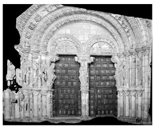
Figure 9: Synthetic image SBA from disparity map. Overlaps almost exactly with image A, but image information comes from image B
