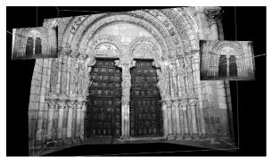
Figure 7: OpenGL "near orthophoto" 3D view. Geometrical depth noise is less noticeable in this view therefore the mesh is adequate
