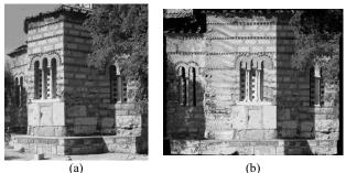
Figure 11: Orthophoto produced with the proposed method (b) using initially "oblique" image (a)
