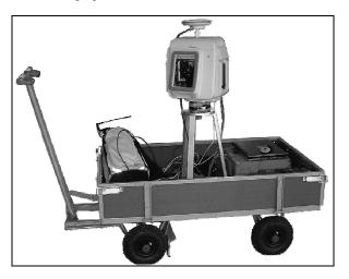
Figure 1: The Trimble® GX scanner integrated on a mobile platform
