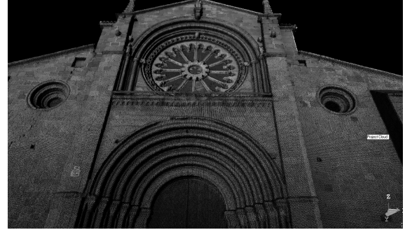
Figure 9: Multi-sensor registration: mapping textures.
