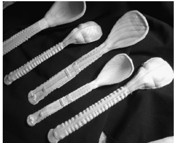
Figure 6: New spoon designs fabricated of wood using a Modela machine.
