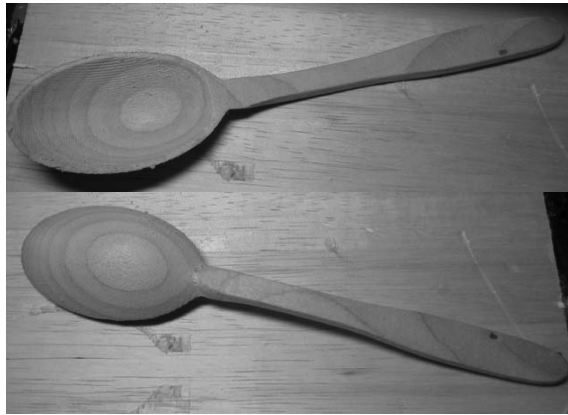
Figure 4: A spoon model fabricated using a Modela machine.
