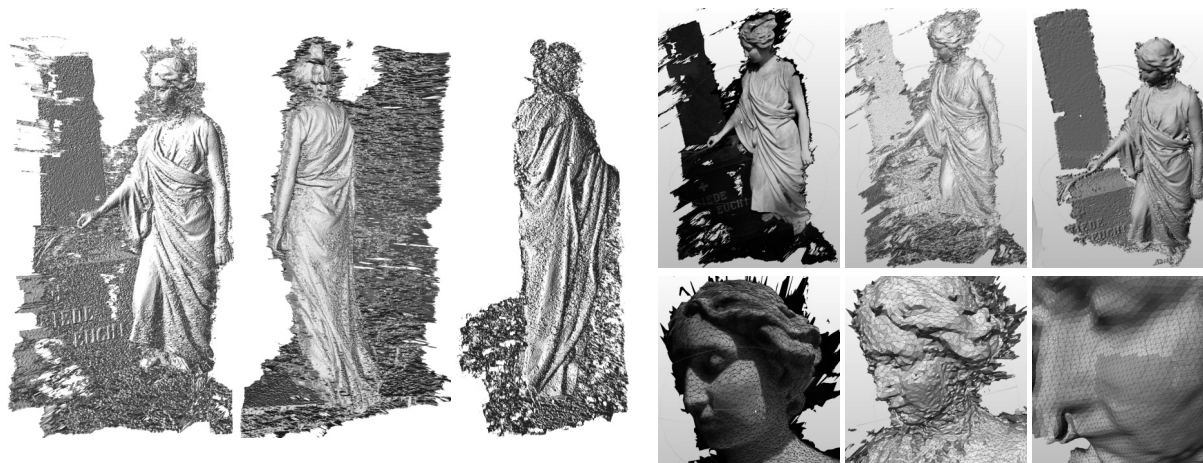
Figure 1: Creating a scanned artifact. Left: Original input data. 3 from 20 noisy range maps are shown un-textured. Right: Simplified versions of the range maps, textured and un-textured. A rectangular region is marked in different triangulations. Rightmost: Several range maps are integrated and smoothed. The gravestone is manually segmented for a semantic markup.
