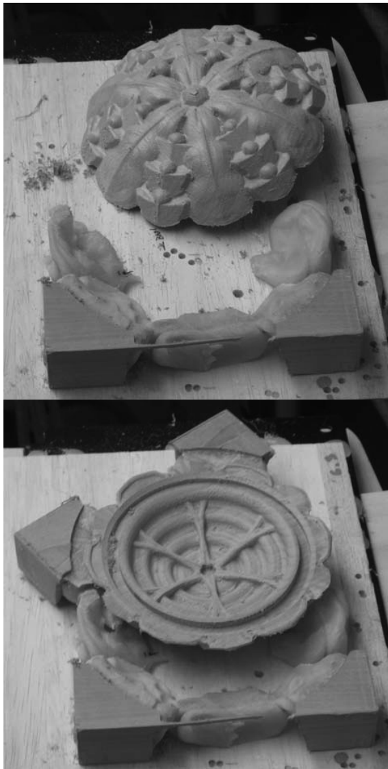
Figure 8: A fabricated wooden bonbonniere lid with tooling for a Modela machine
