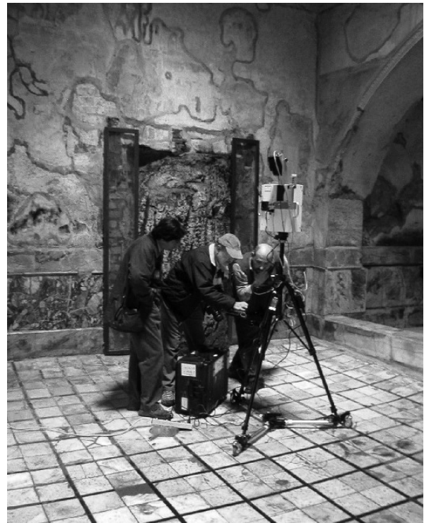
Fig. 3: The laser scanning equipment and some of the survey team at work.
