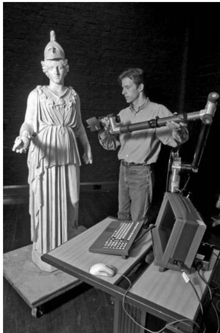
Figure 1: Laser scanning using an arm-mounted sensor.
