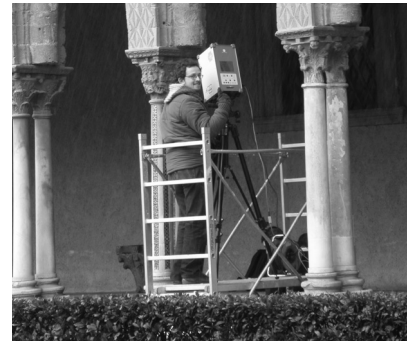
Figure 3: The acquisition setup adopted to scan the capitals.
