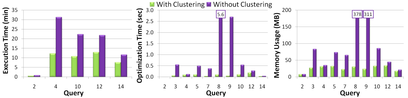
Figure 15: (a) Execution times, (b) Optimization times, (c) Memory usage for enabling and disabling clustering
