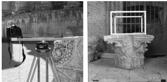
Figure 1: Simple camera bar for stereoscopic exposures with defined base distances of 30 cm and 60 cm (left) and reference frame for stereo model orientation (right)
