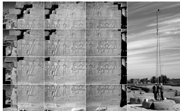
Figure 2: Input 3x4 photo matrix (left), a remotely controlled camera is placed atop a custom vertical rig (right).
