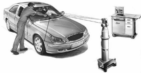
Figure 3: Leica T-Scan laser remotely controlled by the Laser Tracker
