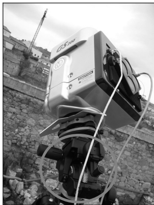
Figure 2: Trimble GS200 laser scanner ( www.trimble.com ) and geared head Manfrotto 400 (red circle).
