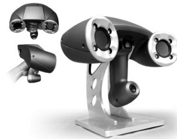
Figure 6: Handyscan 3D: the acquisition unit (980 g, 160 x 260 x 210 mm, ISO accuracy: 20 \mu m + 0.2L/1000)
