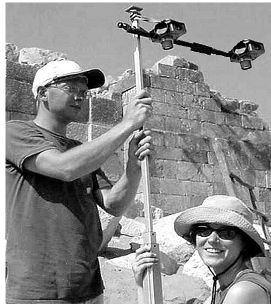
Figure 9: The digital 3D-Rod-Camera Lite with remote control doubtless becomes the most common sensor for extremely close range aerial photography (experimental study)
