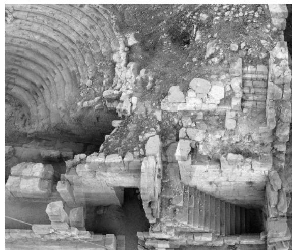
Figure 10: Sample for a low altitude Heritage stereo pair to replace out of date manual sketches (captive balloon 3D view of the Ecclesiasterion in Patara, Turkey; carried out by Dipl.Ing.St.Kiel)
