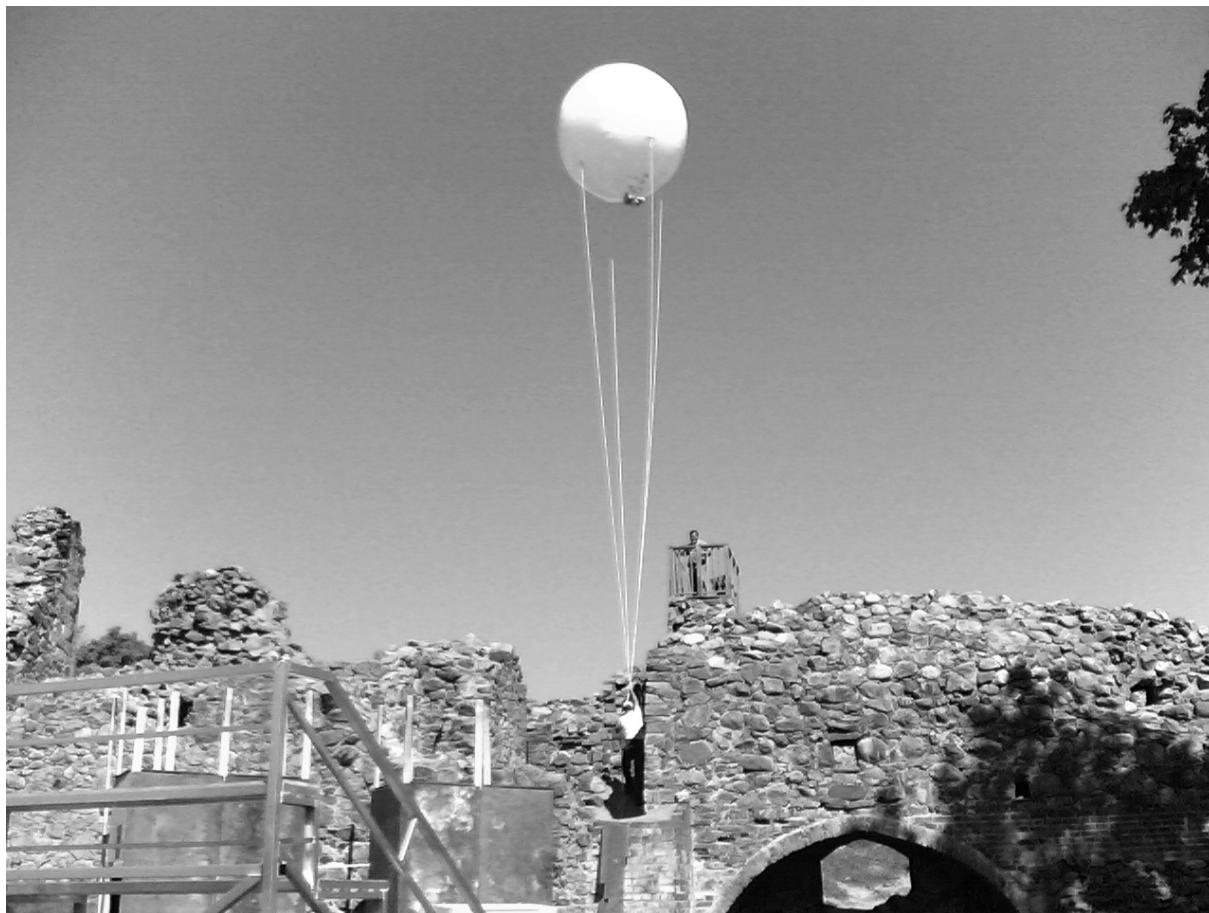
Figure 1: SkyCam 2006 aerial photographic system in use at the Kuusisto Castle in Southwestern Finland
